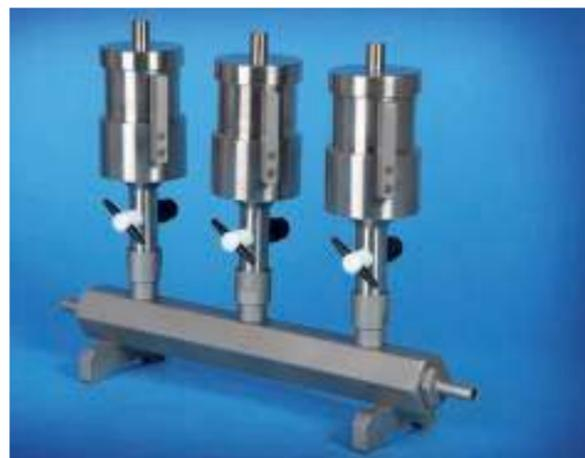
In addition to the single-place filtration device we can also offer stainless steel filtration manifolds. These are ideal for work in benches on account of their compact dimensions.
